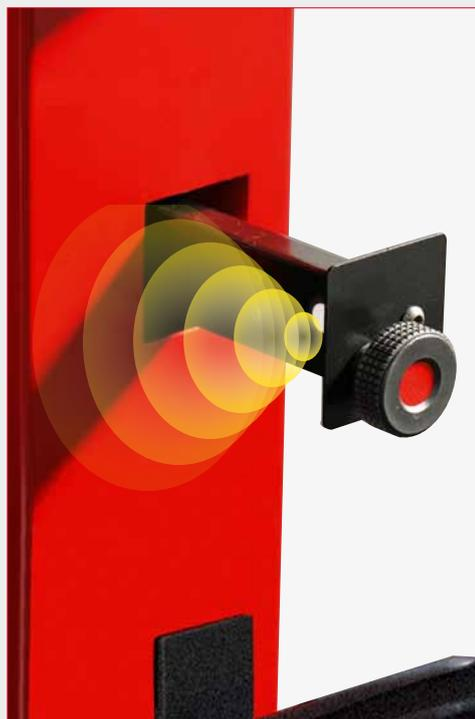
*Diagnosis system for wheel radial run-out that causes vibrations that cannot be fixed with a simple wheel balancing. The presence of the sonar run-out sensor automatically activates the new **BESTFIT** software function which indicates on the screen the point of highest wheel run-out and suggests how to mount it on the hub of the vehicle, before tightening the bolts, in order to eliminate vibrations directly during the assembly on the vehicle.*
