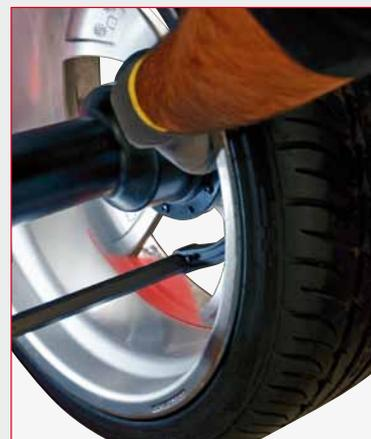
**New digital gauge** for the acquisition of the diameter and distance with the **FSP (Fast Selection Program) function and new integrated LaserBlade pointer**: the FSP function automatically activates the balancing program avoiding selection via the keypad, while the LaserBlade pointer (inside the measuring arm) guides the operator in choosing the level within the alloy rim without any errors and with extremely good visibility.
